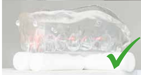
Positioning the scan prosthesis in the CBCT machine on the holder for the test specimen for constancy testing
